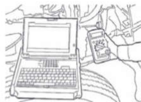
Figure 5. Measuring the Coolant and Air Temperatures
