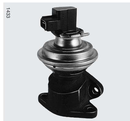
Fig. 3 Exhaust gas recirculation valve with potentiometer position feedback Single-diaphragm type (Diesel engine)
